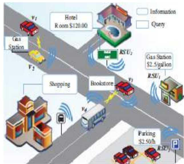
Fig. 1. Future scenario in a vehicle network. Vehicles \{v_1 \dots v_4\} are hearing and storing beacons broadcasted by \{RSU_1 \dots RSU_3\} and opportunistically store-and-forward services information.
