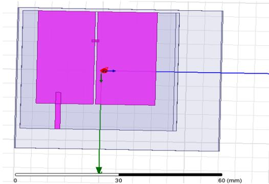
Fig. 4. Patches P1 and P2 are radiating connected using a single PIN diode D1.
