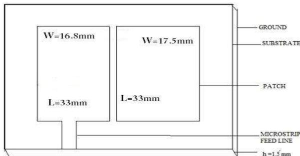
Fig. 1. The proposed geometry of patch antenna
