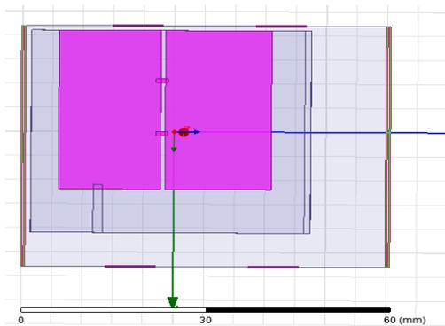
Fig. 5. Patches P1 and P2 are radiating connected using two PIN Diodes D1 and D2.
