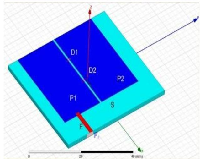
Fig. 2. The designed microstrip rectangular patch antenna.
