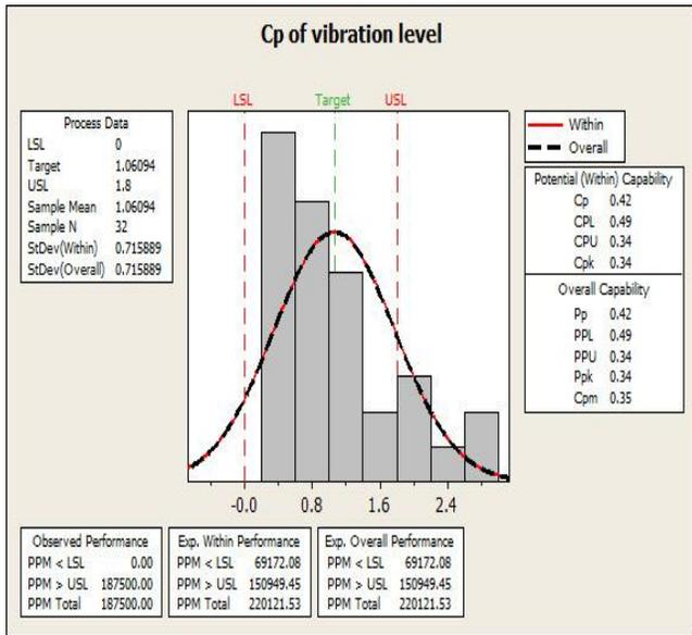
**Fig. 13. Process Capability of Machine 2**
