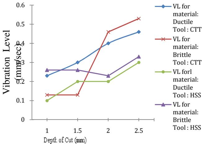
Fig. 2. Vibration Level for Constant Speed.
