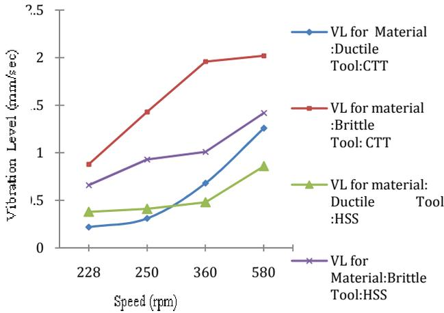
**Fig. 5. Vibration Level for Constant Depth of Cut.**
