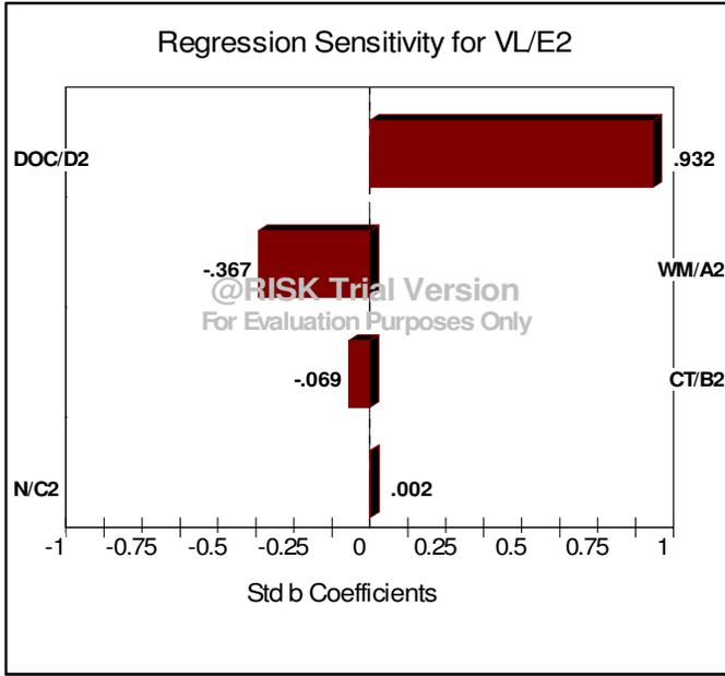
Fig.10. Tornado Graph of Vibration Level
