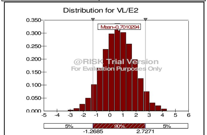
Fig.9. Histogram of Vibration Level
