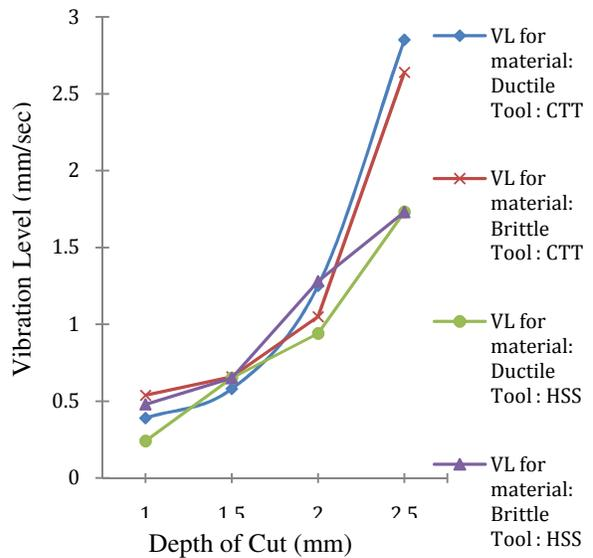
Fig. 4. Vibration Level for Constant Speed
