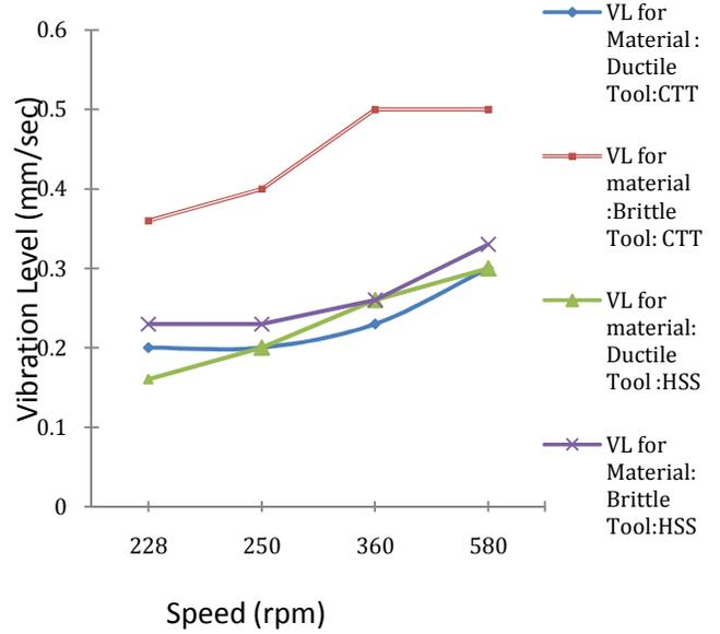
Fig. 3. Vibration Level for Constant Depth of Cut
