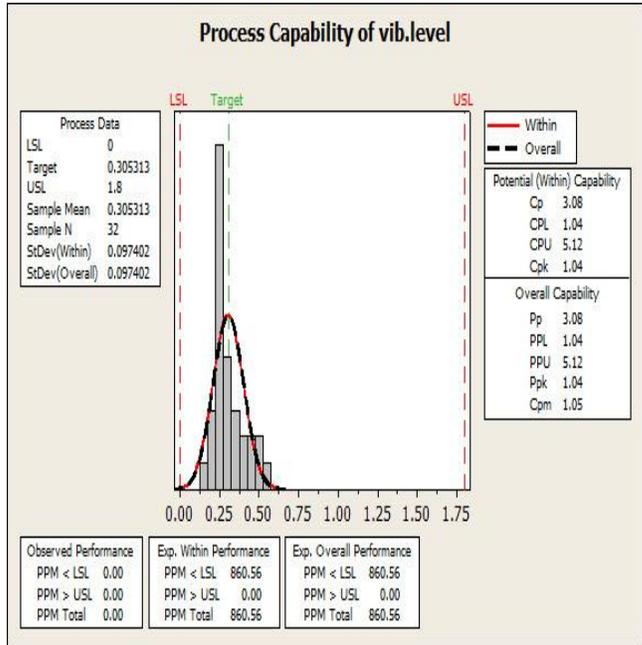
Fig.12. Process Capability of Machine 1
