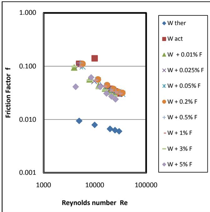
**Fig. 5. Friction factors values for flow of water with different concentration of Flopaam through copper tube**
