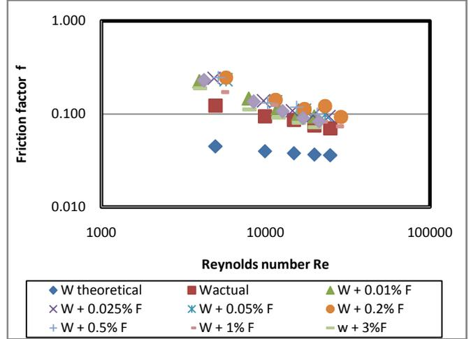
Fig. 3. Friction factor value for flow of water with varying concentration of Flopaam inside Galvanized pipe
