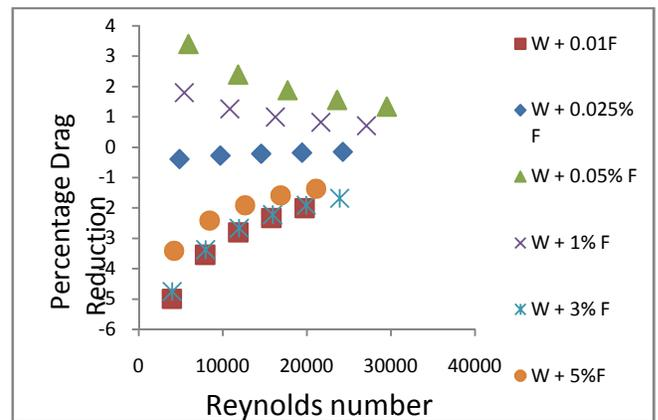
Fig. 4. Percentage Drag Reduction for flow of water with varying concentration of Flopaam through Galvanized Iron pipe
