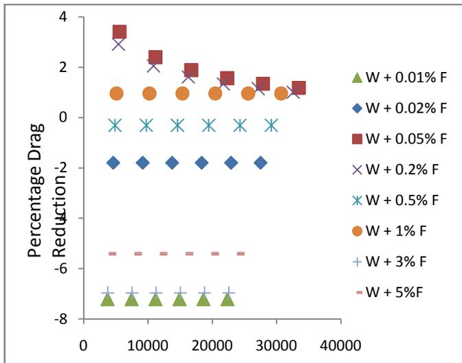
**Fig. 8. Percentage Drag Reduction for flow of water with different concentration of Flopaam through PVC Pipe**
