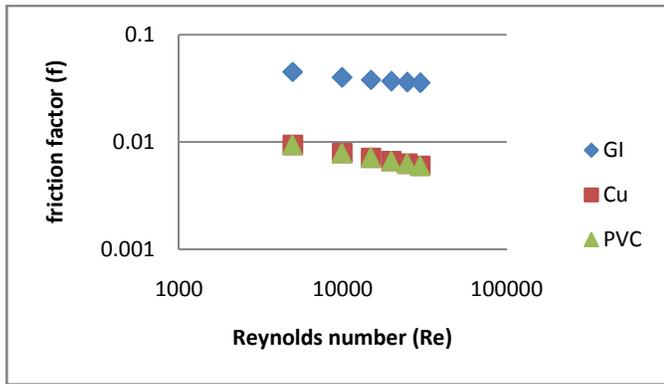
Fig. 2. Friction factor values for varying flow rate of water through Galvanized Iron Pipe, Copper and PVC tubes
