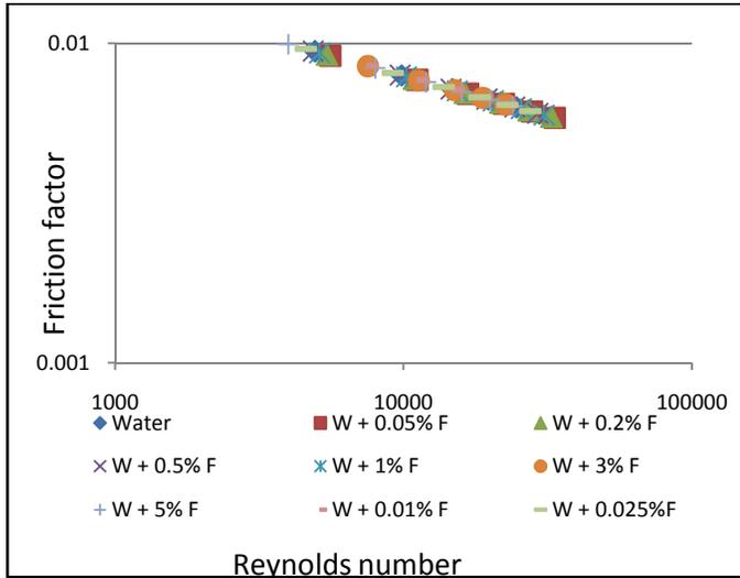
**Fig. 7. Friction factor variation for flow of water with different concentration of Flopaam through PVC Pipe**
