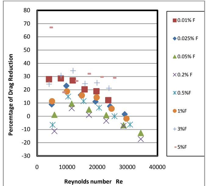
**Fig. 6. Percentage Drag Reduction achieved for flow of water with different concentration of Flopaam through copper tube**
